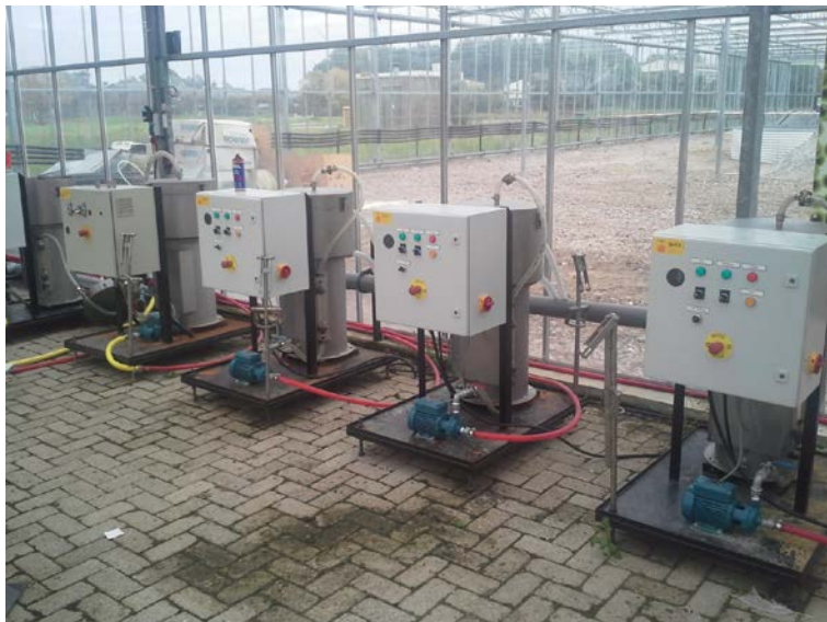
Figure 6. The four centrifuges for harvesting the outside pond.
