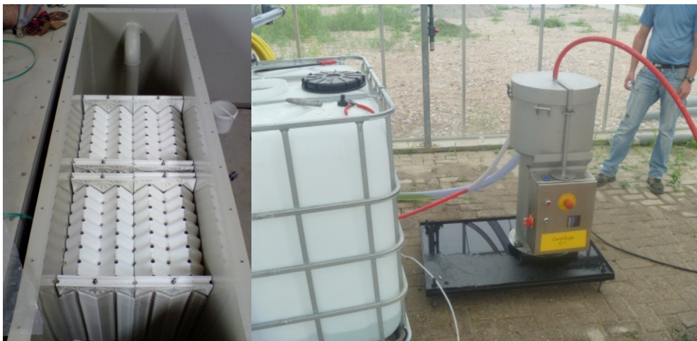
Figure 4. The coalescer (sedimentation tank, left) and the centrifuge (right).
